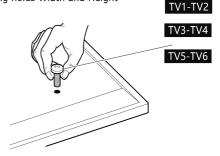
You are provided with 4 diameters of TV fixing screws, **M6** and **M8**. Determine the screw diameter that fits.
