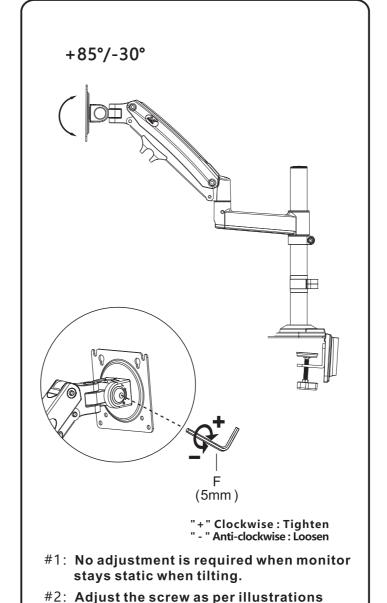
above until monitor stays static at desired angle.
